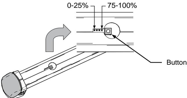
Note the 0-25% indicator flashes when the button is pressed and the battery charge is below 5%.
