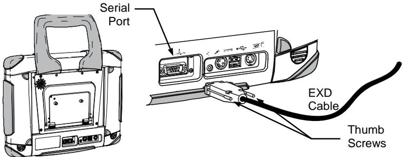
2. Secure the cable connection by tightening the thumb screws.
