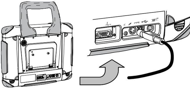
5. Leave the Programmer plugged in until it is fully charged as indicated by the Capacity indicator on the front panel.
